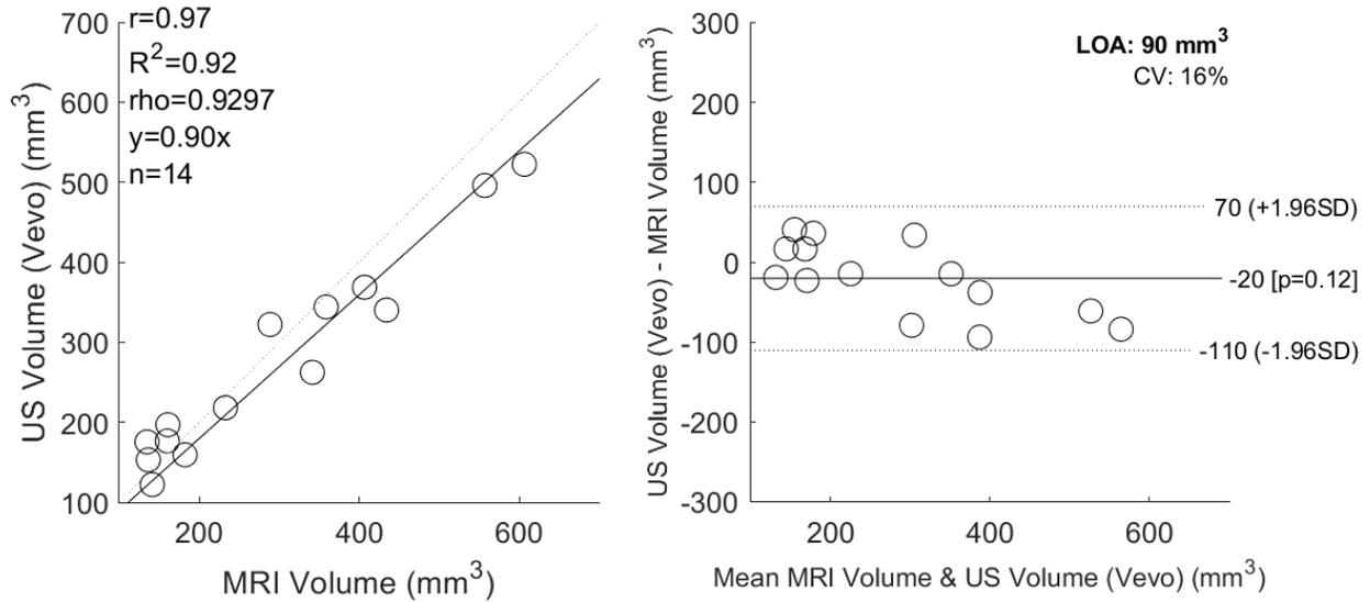
**Regression and Bland-Altman plots comparing *in vivo* measurements of kidney volume between conventional ultrasound to MRI.**  $r$ , Pearson correlation coefficient;  $R^2$ , coefficient of determination;  $\rho$ , Spearman correlation coefficient;  $LOA$ , limits of agreement;  $CV$ , coefficient of variation
