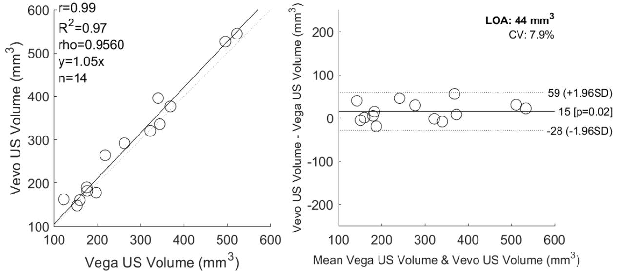
**Regression and Bland-Altman plots comparing *in vivo* measurements of kidney volume between robotic ultrasound to conventional ultrasound (“Vega” and “Vevo” systems, respectively).** *r*, Pearson correlation coefficient;  $R^2$ , coefficient of determination;  $\rho$ , Spearman correlation coefficient; *LOA*, limits of agreement; *CV*, coefficient of variation
